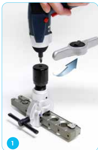
Possibility to operate by manual ratched and electric drill.
