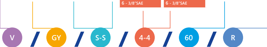
Series GY flexible hose with valve, connections straight-straight, 1/4" x 1/4", 1500 mm, red
